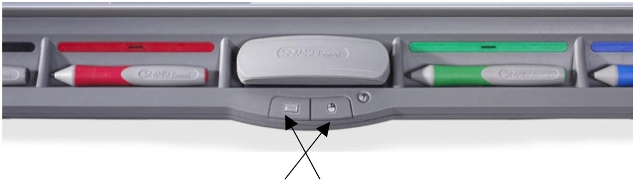
**Press and hold down both buttons on the pen tray at the same time and then release.**
